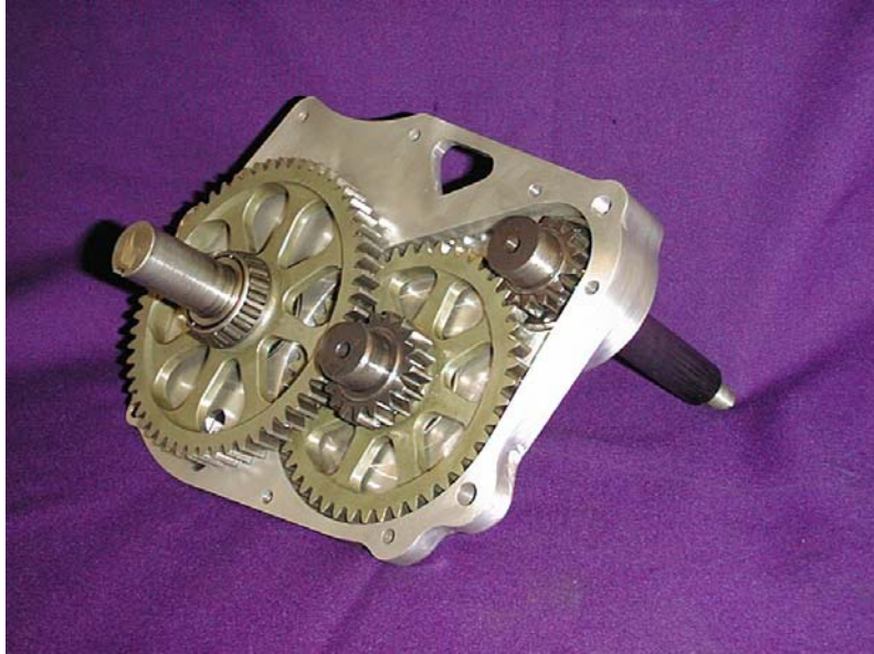
Mini Baja Student Designed and Fabricated Gearbox
