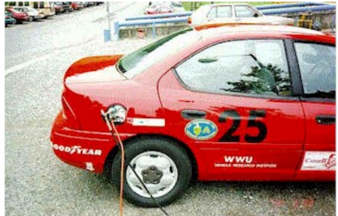
Viking 25 CNG Filament Wound Tank and Converted CNG Filler
