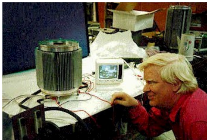
Dr. Fraas with the First TPV Generator to Run a TV
