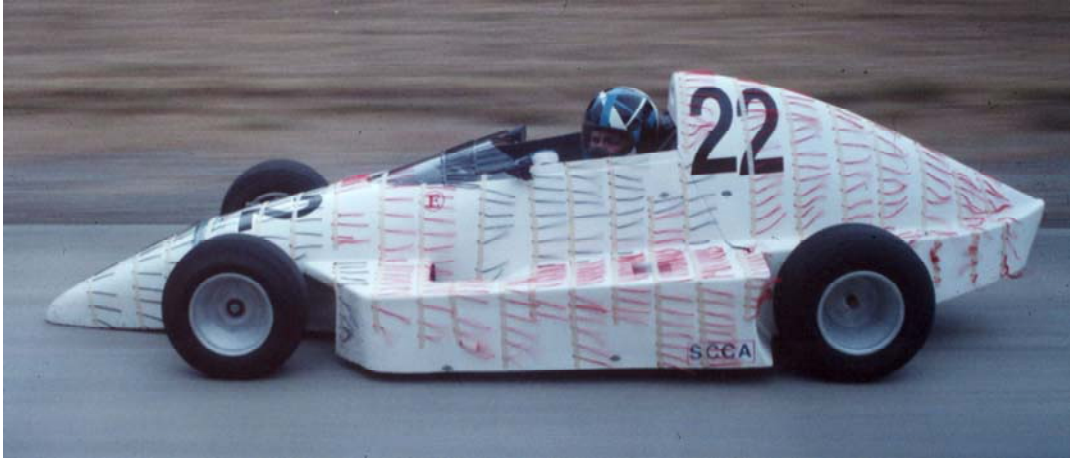
Testing the Aerodynamics of Viking 22
