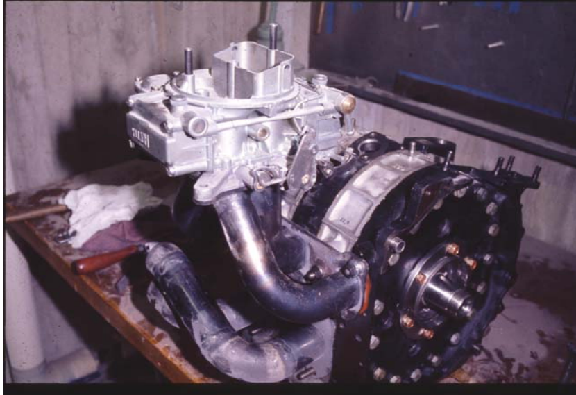
R100 Mazda Rotary with Autolite 600 cfm Four Valve Carburetor
