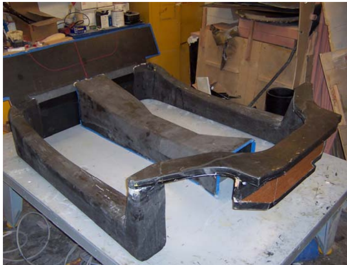
Carbon Fiber Center Chassis
