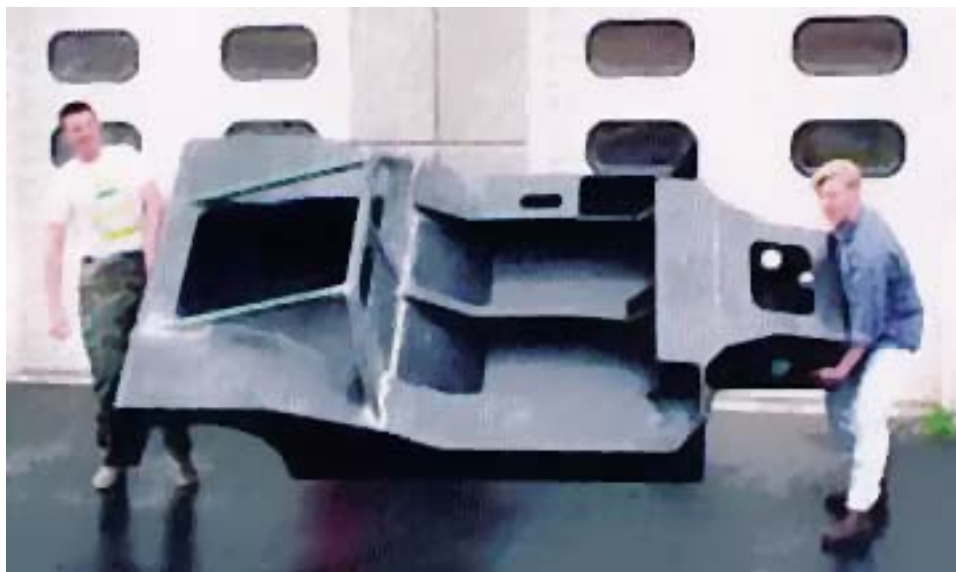
Viking 23's Carbon Fiber Chassis
