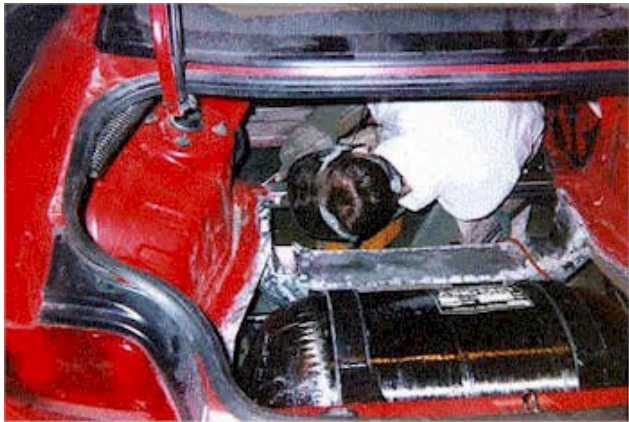
Viking 25 CNG Filament Wound Tank and Converted CNG Filler
