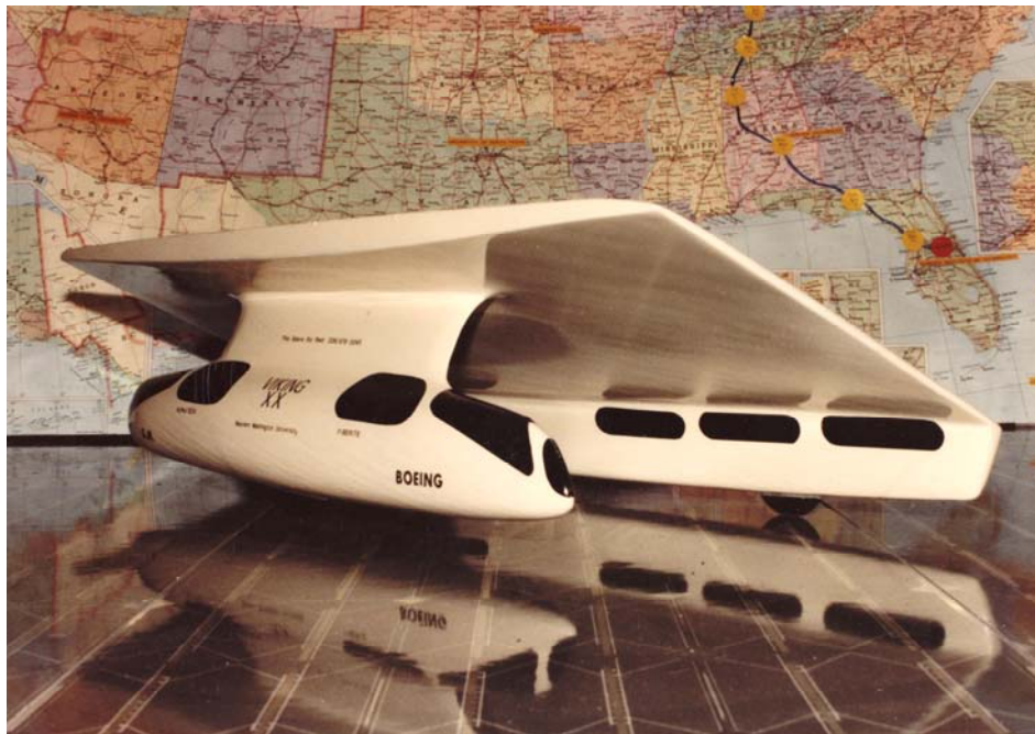
Wind Tunnel Model of Viking XX, Solar Car
